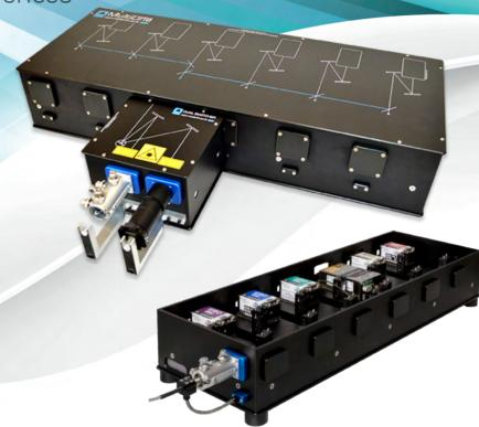
The system can accommodate up to six lasers which can be combined into up to six different fibres with arbitrary light distribution or sharing of wavelengths between ports. Mechanical shutters and galvanometer switching modules are available as required. The lasers can be controlled using the Cairn MultiLine controller with computer and / or front panel digital and analogue modulation, or used with the laser manufacturer or other third-party power supply.
